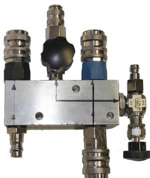
A springloaded exhaust/overpressure valve keeps a constant overpressure of 5mB inside the helmet. This to prevent any return of poisoned gas and/or toxic particles.
